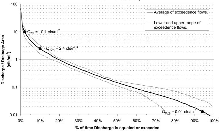
Figure B-6. Regional flow duration curve constructed by averaging the exceedence flows from three stream gaging stations: San Lorenzo Creek above Don Castro Reservoir, Cull Creek above Cull Creek Reservoir, and Castro Valley Creek at Hayward. Error bars represent the minimum and maximum flow associated with the indicated exceedence value.
