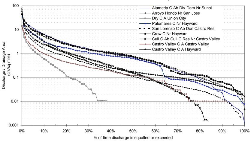
Figure B-4. Flow duration curves constructed using flow data from November through April, the assumed period of steelhead and rainbow trout upstream migration. Note in Table B-2, some of the gage stations have only two years of recorded flows.
