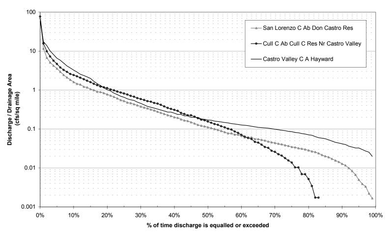
Figure B-5. Flow duration curves constructed using daily average flows from November through April for the three gage sites with the longest record (Dry Creek appears to have regulated flow at times and was excluded).
