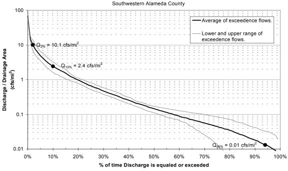
Figure 3.1 – Regional flow duration curve constructed by averaging the exceedence flows from three stream gaging stations: San Lorenzo Creek above Don Castro Reservoir, Cull Creek above Cull Creek Reservoir, and Castro Valley Creek at Hayward. Error bars represent the minimum and maximum flow associated with the indicated exceedence value.
